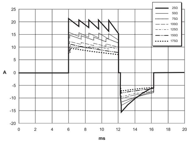
Figure A-4. Rectilinear Biphasic Waveforms at 85 Joules
