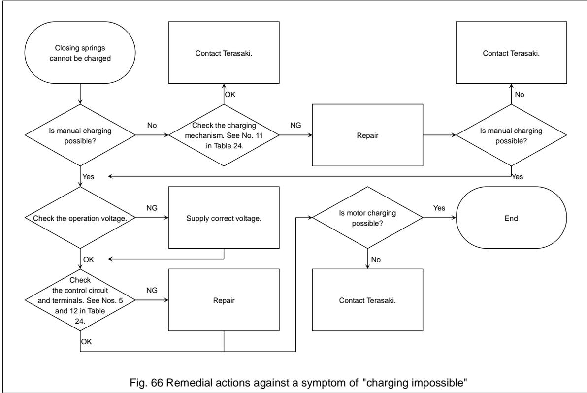
Fig. 66 Remedial actions against a symptom of "charging impossible"
