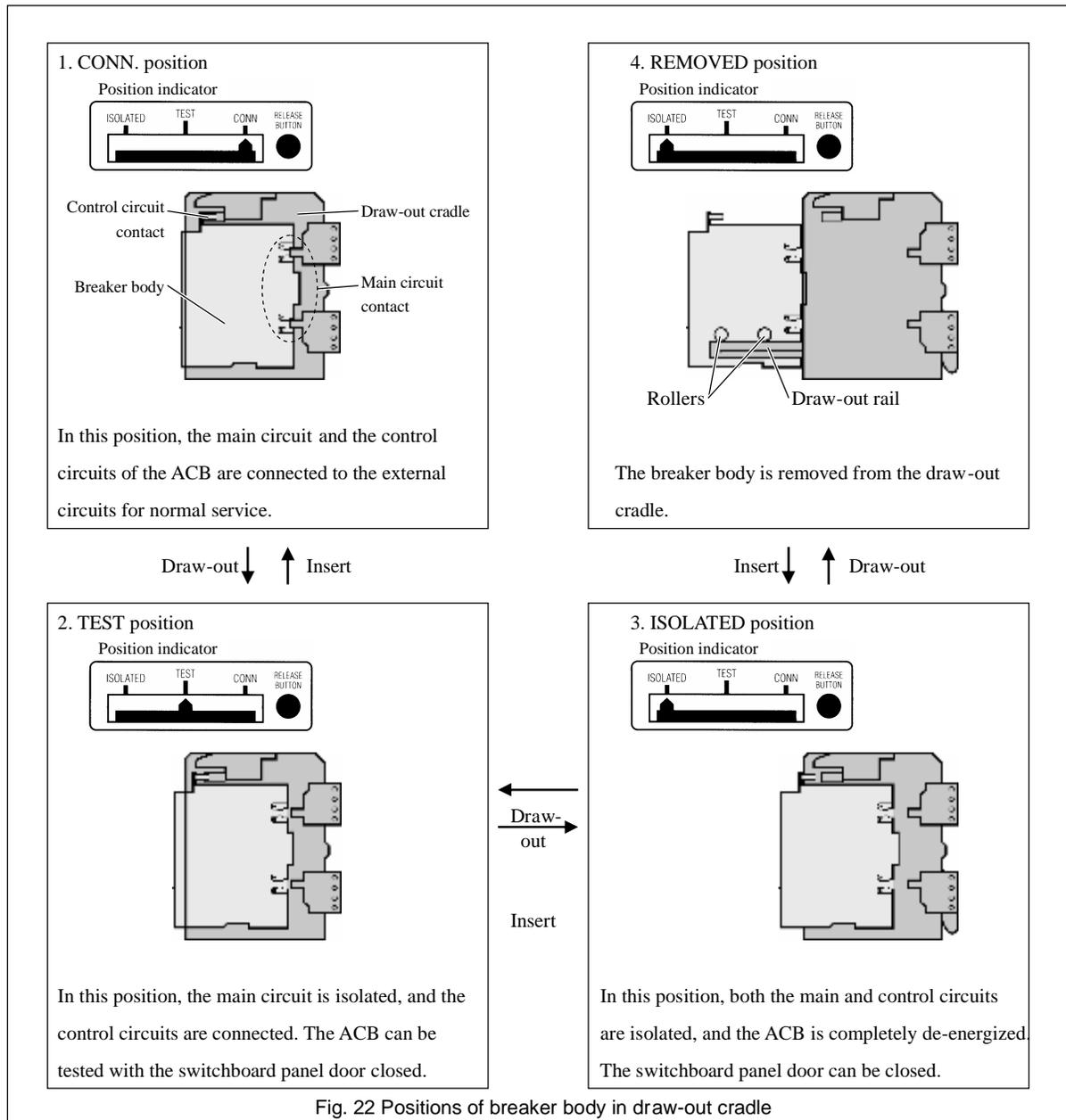
Fig. 22 Positions of breaker body in draw-out cradle
