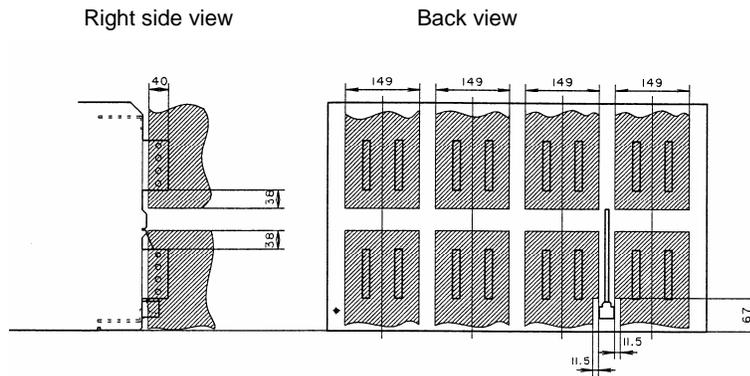
Fig. 7 Conductor (include screw) connection area (AR440S)
