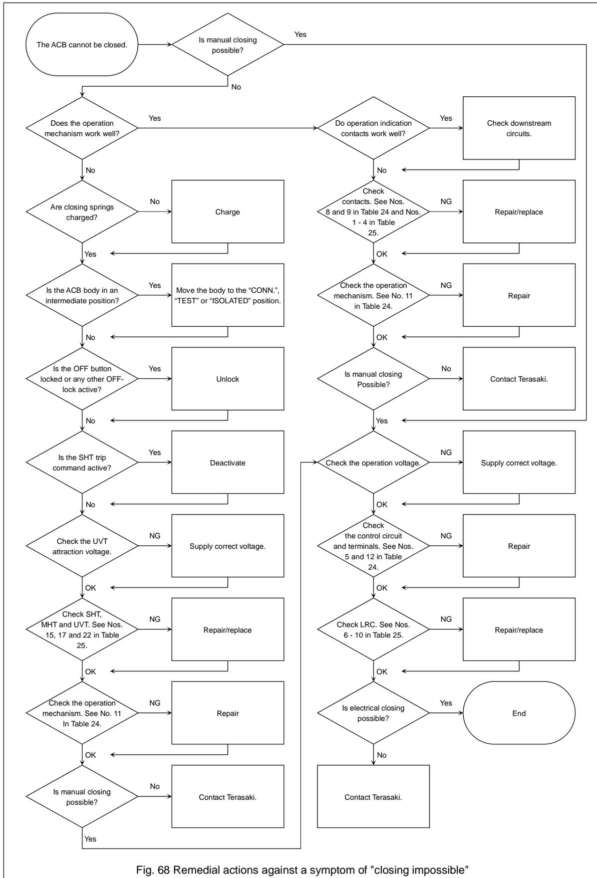
Fig. 68 Remedial actions against a symptom of "closing impossible"
