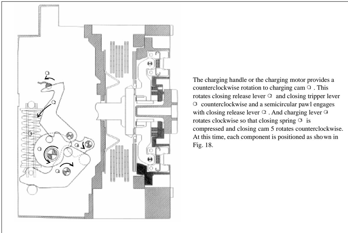
The charging handle or the charging motor provides a counterclockwise rotation to charging cam Q . This rotates closing release lever Q and closing tripper lever Q counterclockwise and a semicircular pawl engages with closing release lever Q . And charging lever Q rotates clockwise so that closing spring Q is compressed and closing cam 5 rotates counterclockwise. At this time, each component is positioned as shown in Fig. 18.
