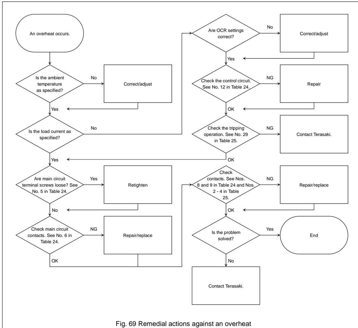
Fig. 69 Remedial actions against an overheat
