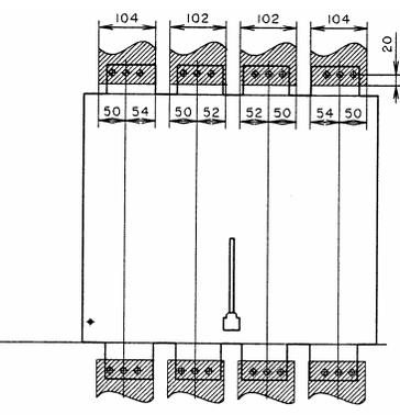
Fig. 6 Conductor (include screw) connection area (AR325S, AR332S, AR316H, AR320H, AR325H, AR332H)
