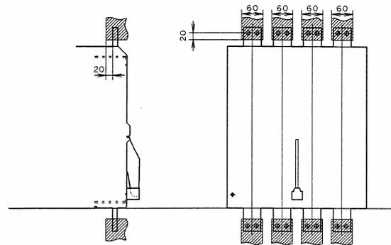
Fig. 5 Conductor (include screw) connection area (AR208S, AR212S, AR216S, AR220S, AR212H, AR220H)
