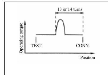
Fig. 25 Handle operating torque
