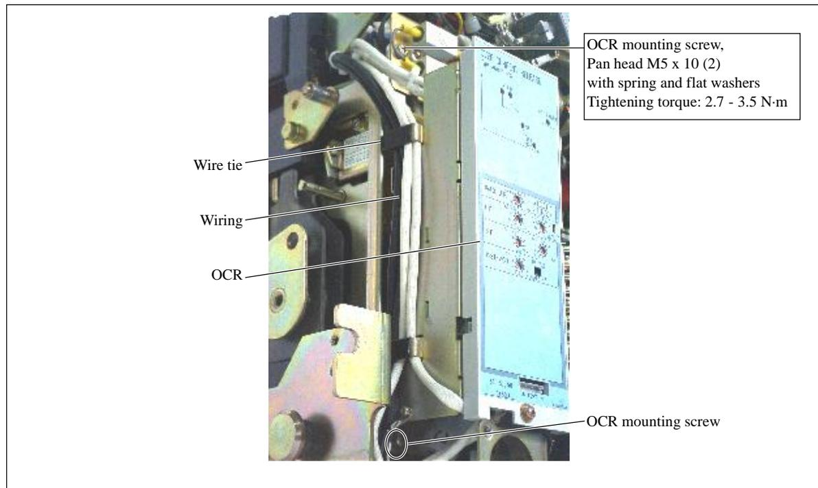
6) Pull out the OCR as shown in Fig. 57 and place it on the floor.
