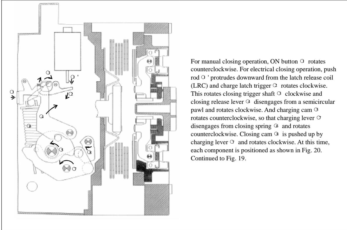
Fig. 18 Closing motion 1 (discharge motion)
