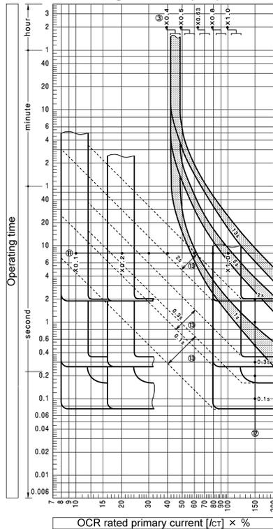
N-phase protection trip and ground fault trip
