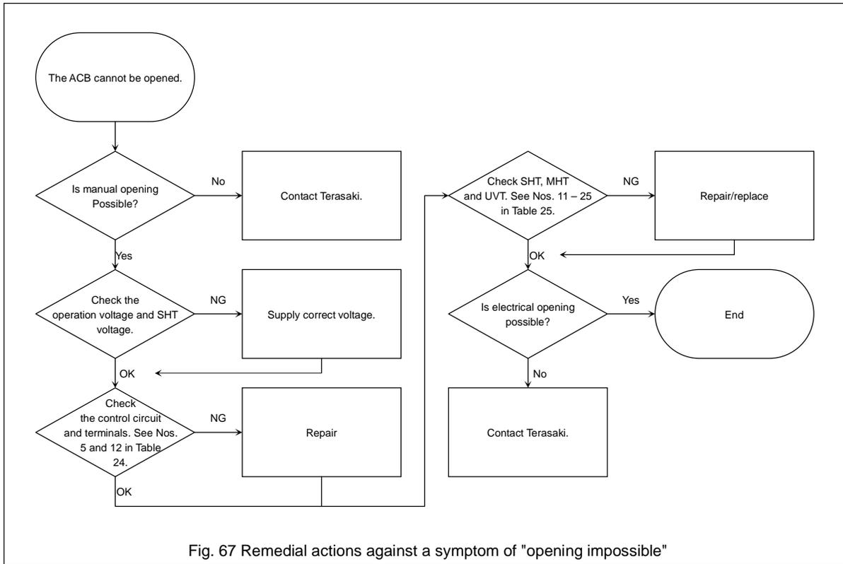
Fig. 67 Remedial actions against a symptom of "opening impossible"
