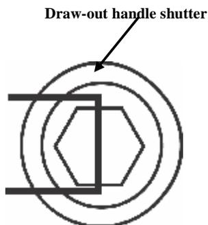
The handle shutter is a good position at the centre of the hole and no adjustment is required
