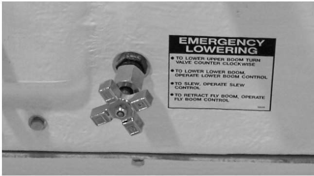
Figure 8.9 - Insulated Fibreglass Basket, Emergency Lower Valve
