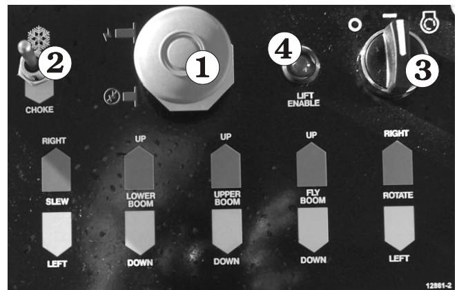
Figure 8.5 - Upper Control Box Controls - Steel Basket
