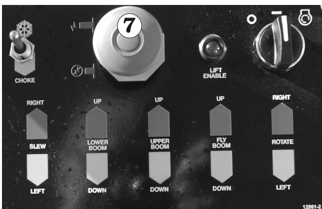
Figure 9.25 - Platform Control Switches - Steel Platform
