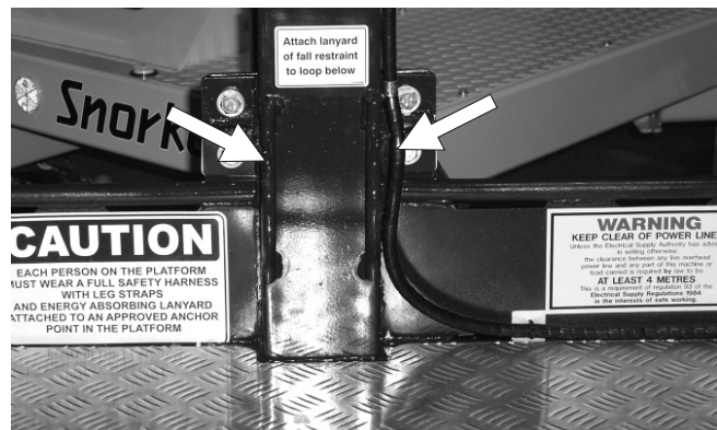
Figure 9.14 - Lanyard Anchor Points - Steel Platform
