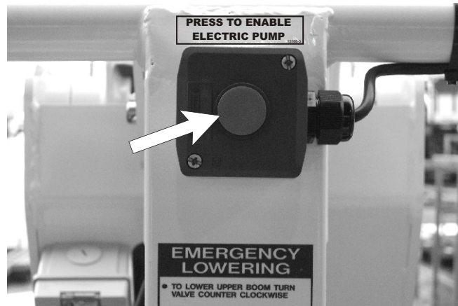
Figure 13.5.2 - Electric Motor Enable Switch Platform Station, Hydraulic Controls
