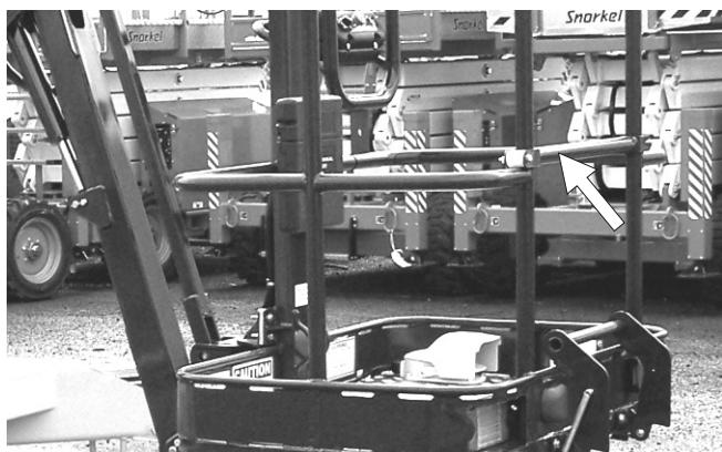
Figure 9.15 - Platform Gravity Gate
