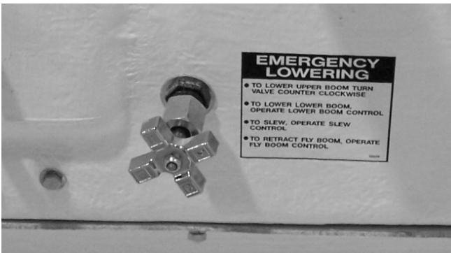
Figure 8.12 - Emergency Lower Valve - Non-Insulated Fibreglass Basket
