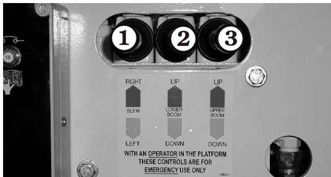
Figure 8.4 - Lower Controls - Movement Control Valve Levers
