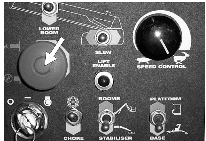
Figure 10.1 - Ground Control Box Emergency Stop Switch Location.
