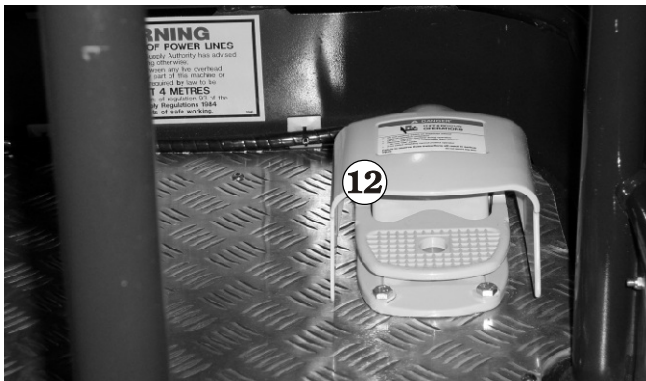
Figure 7.5 - Upper Controls - Foot Switch
