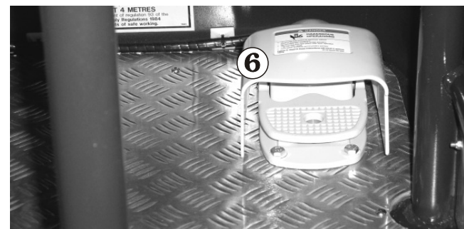
Figure 10.16 - Platform Foot Switch
