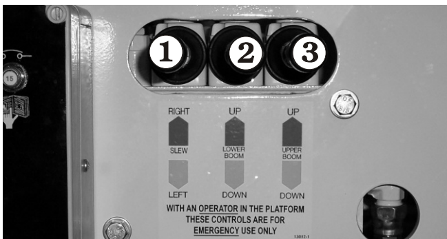
Figure 10.18 - Movement Control, Ground Control Box
