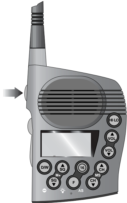
Fig 2.6 - Switching On and Off
