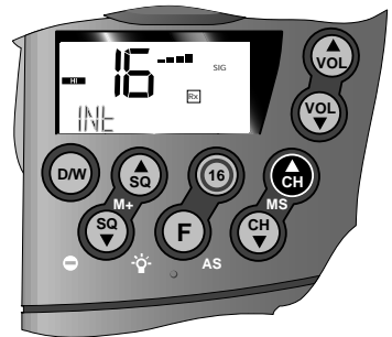
Fig 2.8 - Squelch bargraph on LCD display
