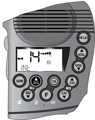
Fig 2.8 - Squelch bargraph on LCD display
