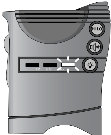
Fig 2.5 - Rx LED: receiving, fully squelched
