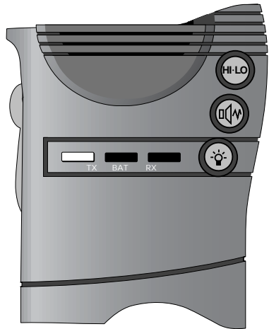
Fig 2.4 - Tx LED: transmitting on high power
