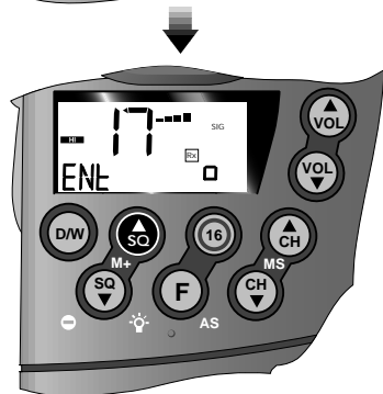
Fig 2.11 - Entering channel into Scan Memory
