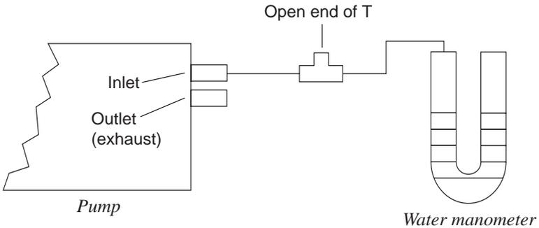
2. On the open end of the "T," draw vacuum by mouth until 4 to 5 inches of water vacuum register on the manometer.
