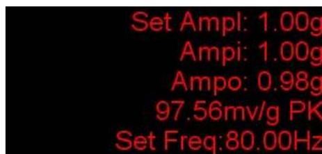
The first line (Set Ampl) indicates the specified vibration amplitude; the second line (Ampi) indicates the actual vibration amplitude; the third line (Ampo) indicates the actual vibration amplitude of external sensor; the fourth line indicates the actual sensitivity of external sensor and measurement type (PK or RMS); the fifth line (Set Freq) indicates the specified working frequency.
