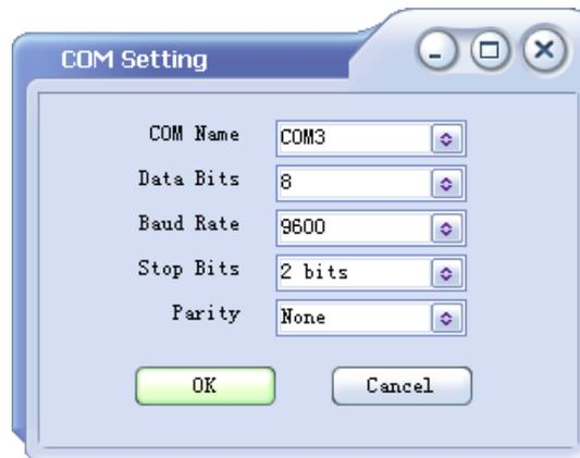
Set correct communication parameters on “COM Setting” window, and then click **OK** button, later click **Reset** button to re-connect to the PT520 device.
