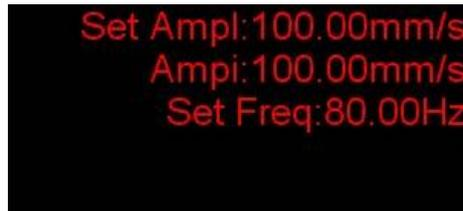
The first line (Set Ampl) indicates the specified vibration amplitude; the second line (Ampi) indicates the actual vibration amplitude; the third line (Set Freq) indicates the specified working frequency.
