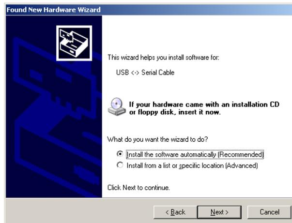
3. The computer now begins to scan the installation file and then install the USB-RS232 converter driver.
