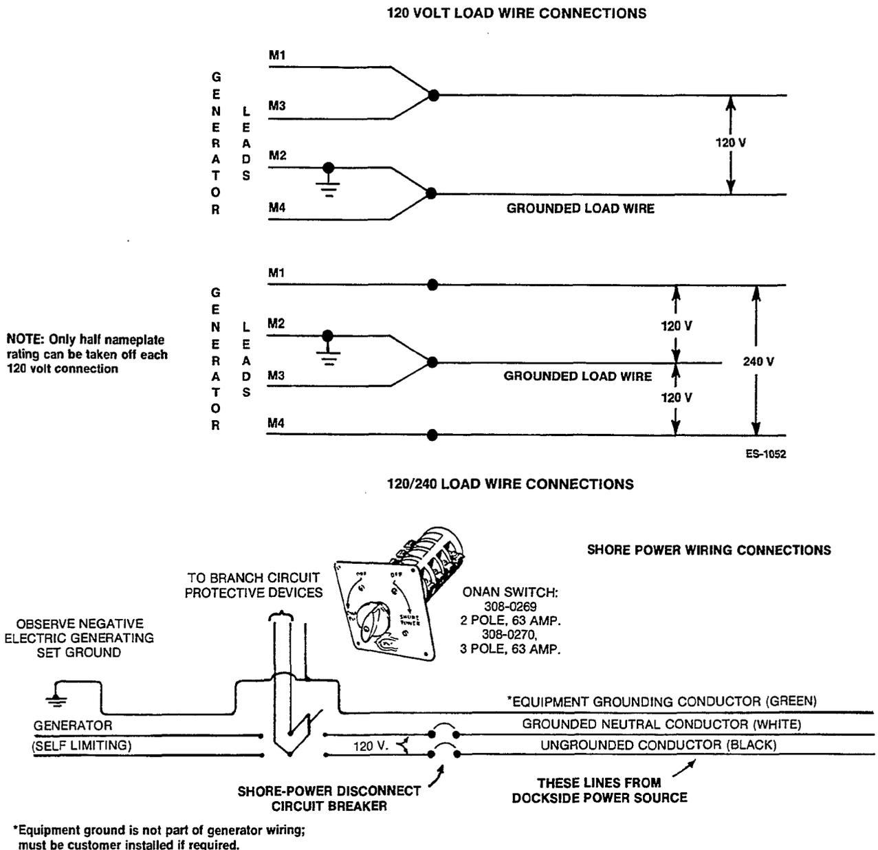
FIGURE 15. LOAD WIRE CONNECTIONS
