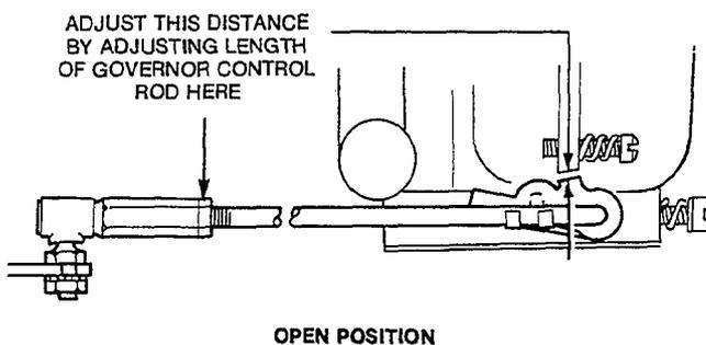
**FIGURE 22. LINKAGE ADJUSTMENT**
