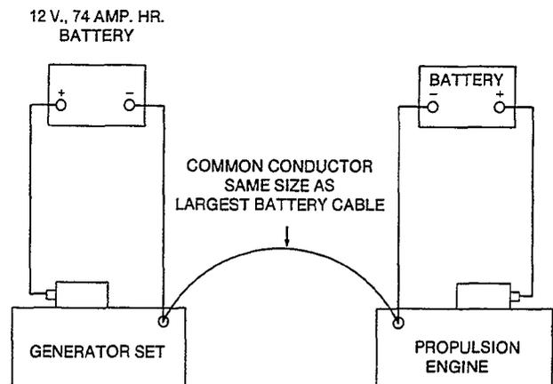
FIGURE 13. BATTERY CONNECTIONS
