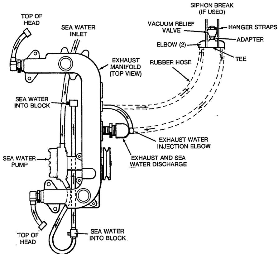
FIGURE 10. HOSE SCHEMATIC, SEA WATER COOLING
