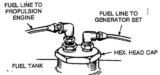
FIGURE 5. TWO FUEL LINES IN ONE TANK OUTLET
