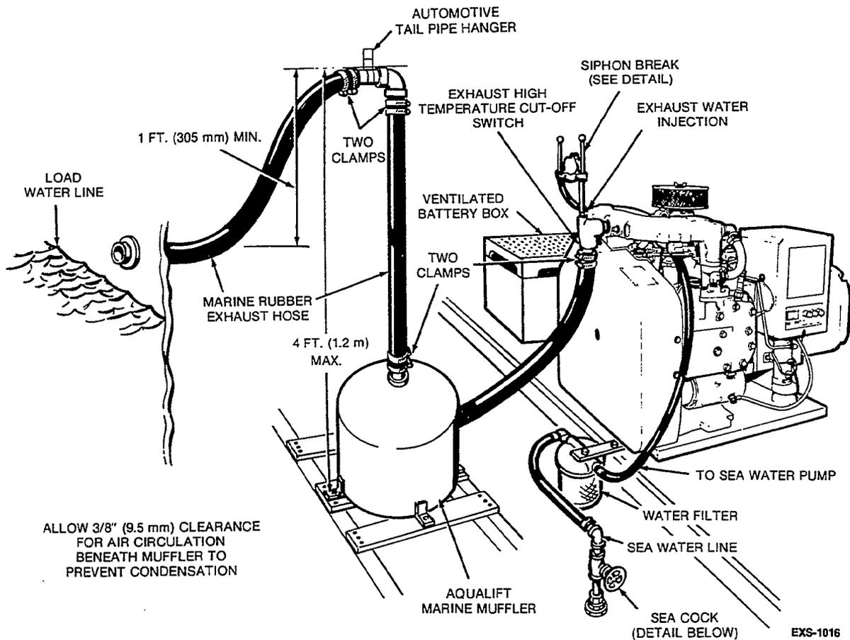
**CAUTION** Install Siphon Break Kit #155-0950 if exhaust injection elbow is below load water line. Locate the Siphon Break at least 12 inches (305 mm) above load water line and in a vertical position. Remote mounting the siphon break is permissible within a 5 foot (1.5 m) radius of water injection exhaust elbow. Vertical position and height of valve must be maintained.
