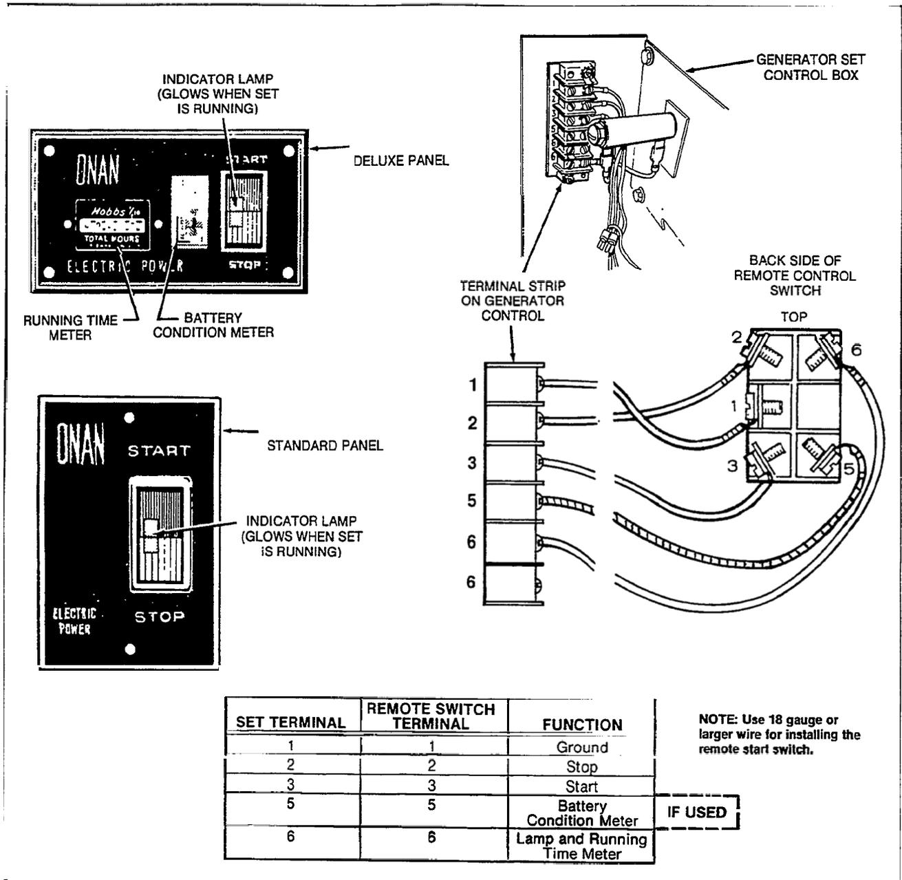
FIGURE 14. WIRING CONNECTIONS FOR REMOTE CONTROLS
