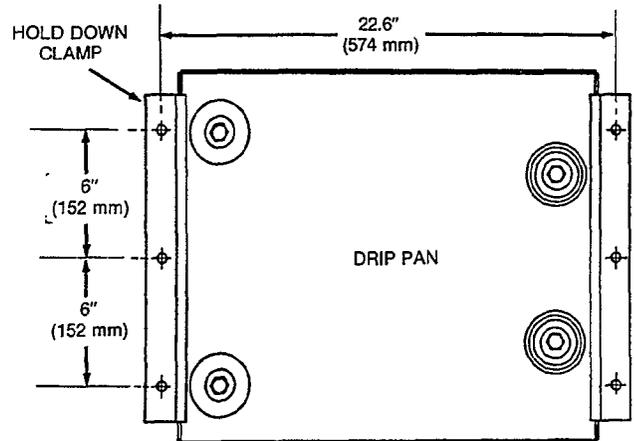
FIGURE 1. MOUNTING DIMENSIONS
