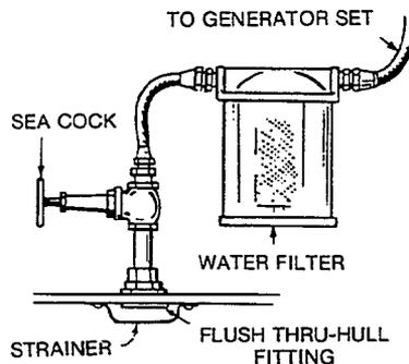
**CAUTION** Do not use scoop type water inlet fittings on generator sets using Aqualift muffler systems.
