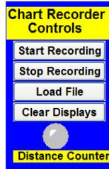
**Data acquisition** is started, and both chart recorders in a panel are turned on by pushing the **Start Recording** button. Recording is stopped by pushing **Stop Recording**.
