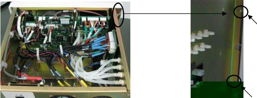
3. Disconnect the data line from the 7" display conversion board. Peel the fiber adhesive tape fastening the data line. Note: when disconnecting the data line, you must push out the black holder parallel to the conversion board.
