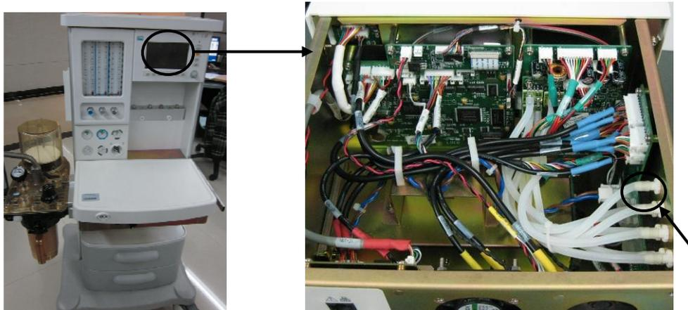
5. Disconnect the cables from the power board, network conversion board and calibration power interface board.
