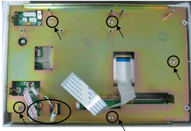
5. Peel the fiber adhesive tape fastening the data line. Disconnect the data line from the 7" display to remove the display. Note: when disconnecting the data line, you must lift the black fixer.
