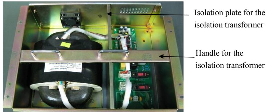
2. Disconnect the three cables from the drive board for the isolation transformer. Unplug the connector to the fan connection line. Unscrew the four screws as shown below to remove the isolation transformer.
