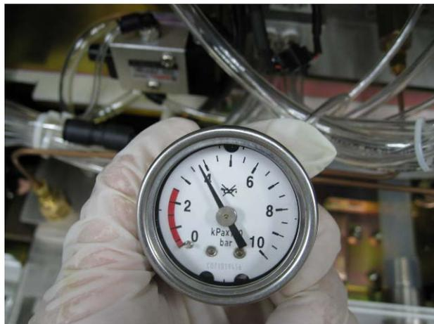
9. Turn on the pipeline gas supply and record the reading on the test pressure gauge. If the difference between this reading and the reading on the O2 pipeline pressure gauge is more than 0.1 MPa (1 bar), it indicates that the O2 pipeline pressure gauge is damaged. Handle this problem as described in the troubleshooting table.
