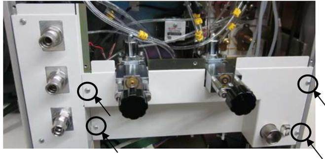
3. Disconnect the tubes from the high pressure cylinder yoke. Remove the connector connected to the yellow copper tube. Unscrew the five screws as shown below to remove the cylinder yoke support (with cylinder yoke).
