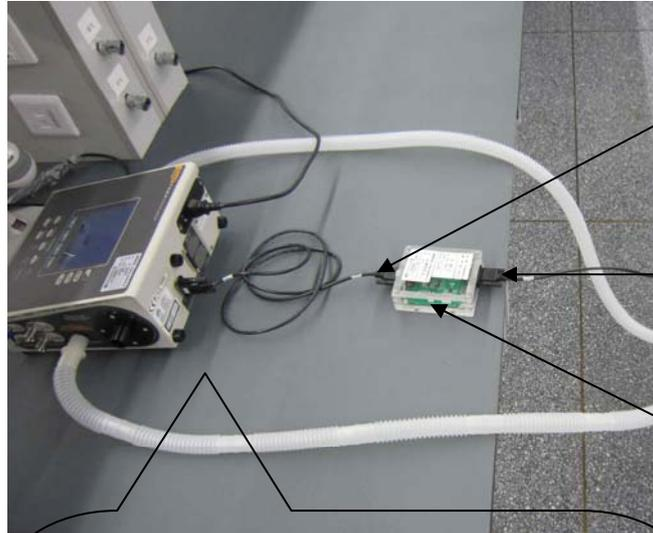
RS232 connection line to the calibration device
