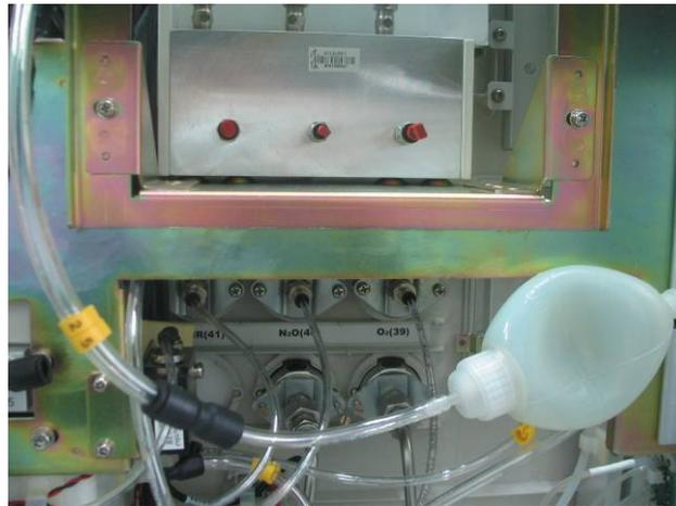
7. Release the negative pressure ball. If the negative pressure ball is fully expanded within 30s, it indicates that the flowmeter is damaged. Handle this problem as described in the troubleshooting table.
