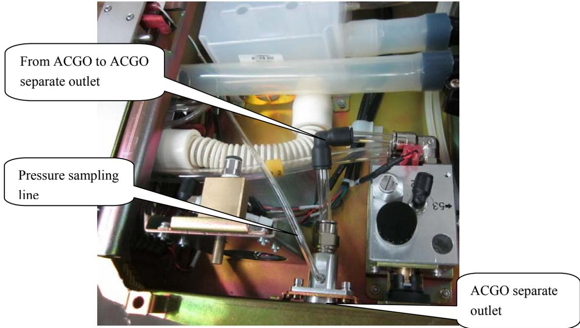
When ACGO is turned on, the anesthesia machine stops mechanical ventilation. The fresh gas is directly outputted through the inspiration connector on the breathing circuit. Pressure relief valve 53 on the ACGO prevents pressure at the ACGO port from exceeding 110cmH<sub>2</sub>O when ACGO is turned on.
