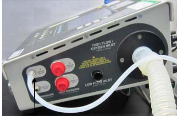
Fluke VTPlus pressure sampling connector (high pressure)
