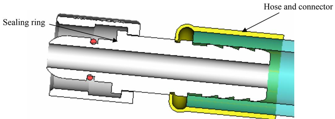
If any damage or loose connection is detected, replace the corresponding part.
