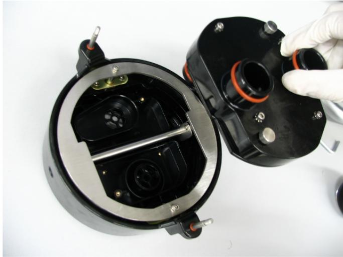
8. Pull up to take out the lifting device.
