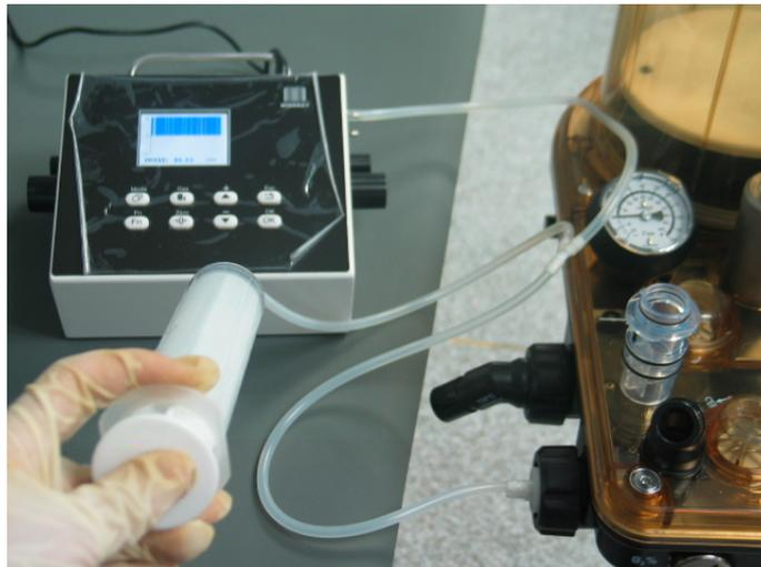
6. Push in the push rod of the injector to let the pressure reading on the anesthesia machine calibration device rise to 70 to 90  $\text{cmH}_2\text{O}$  and then stop pushing. Keep the relative position between the push rod and the injector unchanged. If the pressure reading on the anesthesia machine calibration device does not fall more than 5 $\text{cmH}_2\text{O}$  within 15 s, this test is passed.
