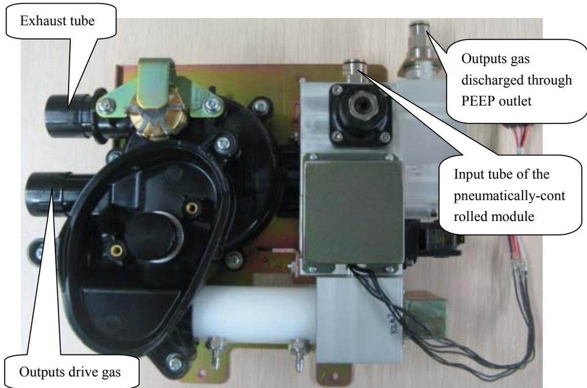
The following figure shows the pneumatic circuit of the pneumatically-controlled module.
