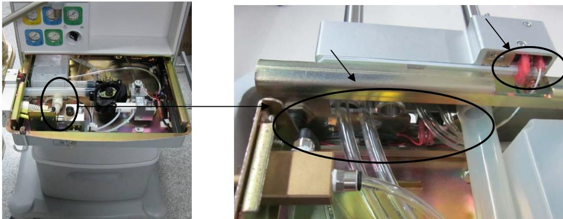
4. Unscrew the four screws as shown below to remove the circuit adapter.
