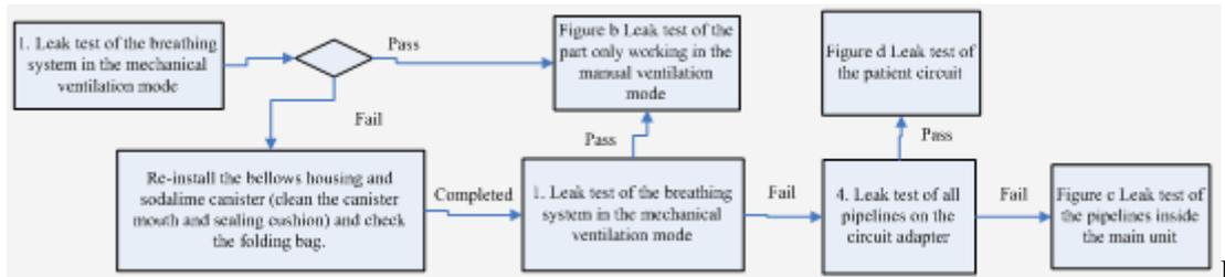
Figure a System leak test
