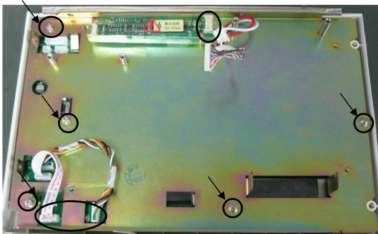
4. Unscrew the four screws as shown below to remove the display.
