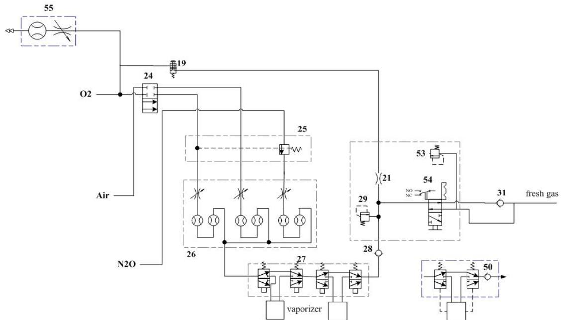
The following picture takes O<sub>2</sub>+N<sub>2</sub>O+Air configuration as an example to illustrate how pipeline supplies are outputted. O<sub>2</sub> is divided into two pathways. One pathway of O<sub>2</sub> flows into system switch 24 and the other into O<sub>2</sub> flush valve 19. N<sub>2</sub>O flows into O<sub>2</sub>-N<sub>2</sub>O cut-off valve 25 and Air into system switch 24.
