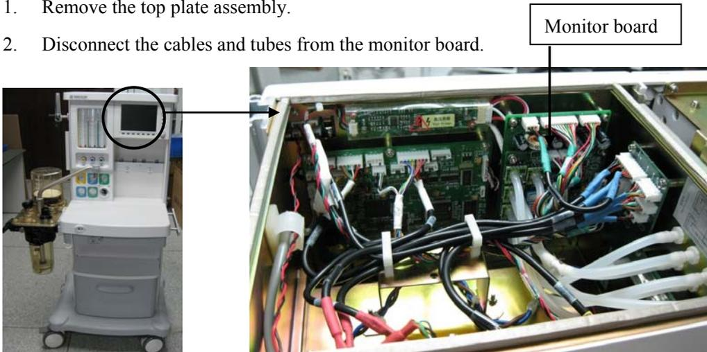
3. Unscrew the two screws as shown below to remove the monitor board.
