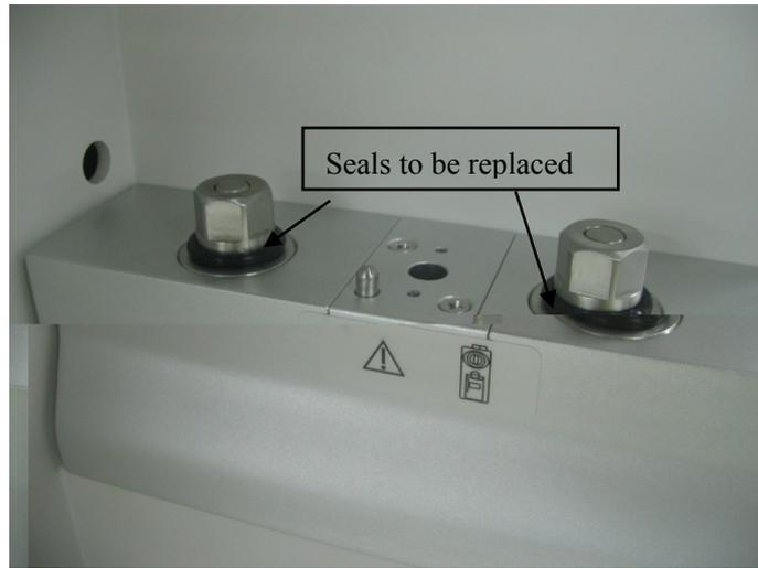
3. As required, replace the seal for valve cover (M6M-010031--) and valve seal (M6M-010033---) every 12 months.
