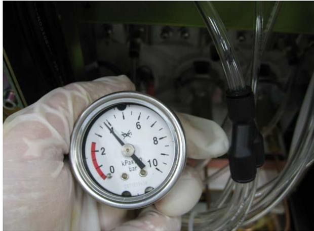
8. Turn on the N<sub>2</sub>O pipeline supply and record the reading on the test pressure gauge. If the difference between this reading and the reading on the N<sub>2</sub>O pipeline pressure gauge is more than 0.1 MPa (1 bar), it indicates that the N<sub>2</sub>O pipeline pressure gauge is damaged. Handle this problem as described in the troubleshooting table.
