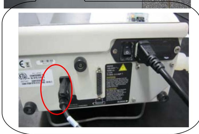
RS232 connection line at the end of calibration device (VT Plus)
