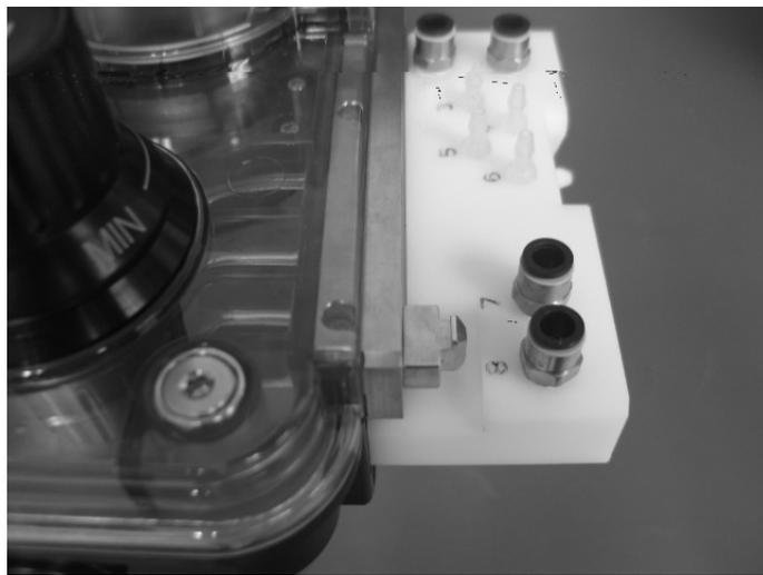
If it is hard to plug in and out the test fixture, apply a layer of KRYTOX lubricant (BOM number: M6F-020003---) to the seals (as shown below).
