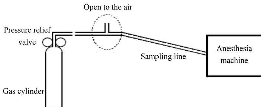
7. Vent the sampling line to CO<sub>2</sub> opening the cylinder pressure relief valve.
