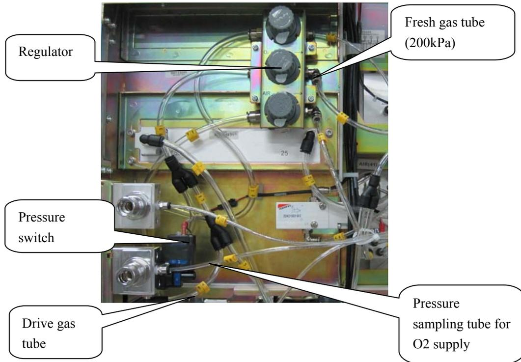
The following picture shows the output connector of cylinder supply inlet assembly.
