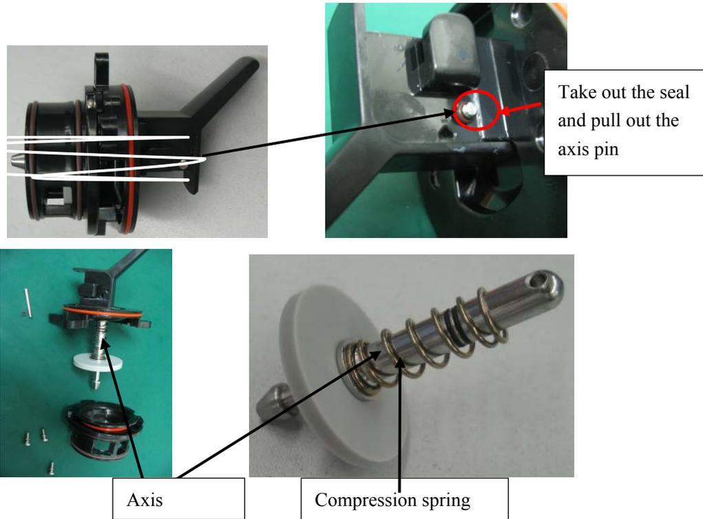
5. Remove the compression spring and replace the two seals (0030-10-13077).
