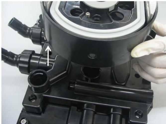
6. Turn over the lifting device. Loosen the two screws as shown below by using the allen wrench.
