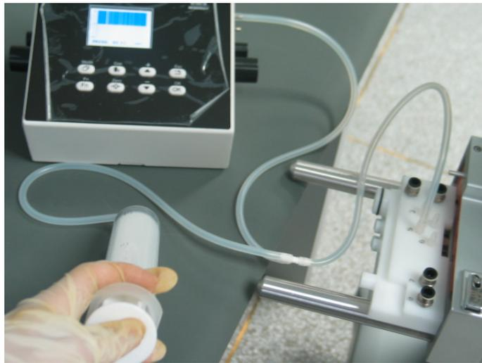
3. Push in the push rod of the injector to let the pressure reading on the anesthesia machine calibration device rise to 70 to 90 cmH<sub>2</sub>O and then stop pushing. Keep the relative position between the push rod and the injector unchanged. If the pressure reading on the anesthesia machine calibration device does not fall more than 5 cmH<sub>2</sub>O within 15s, this test is passed.
