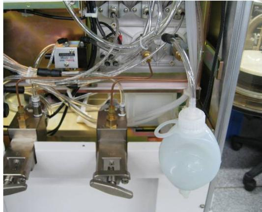
6. Release the negative pressure ball. If the negative pressure ball is fully expanded within 30s during one of the three tests, it indicates that the O<sub>2</sub>-N<sub>2</sub>O cut-off valve assembly is damaged. Handle this problem as described in the troubleshooting table.
