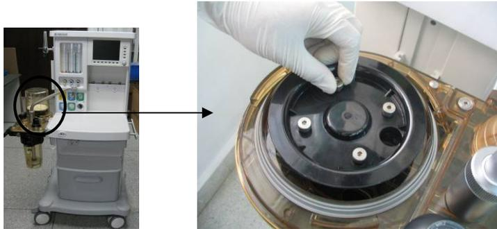
3. Hold and pull up the Pop-off valve cover to remove it.
