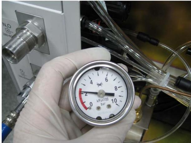
4. Turn on O2 pipeline supply and record the reading on the O2 pipeline pressure gauge. Observe the test pressure gauge. If the reading on the test pressure gauge is not within the range of 0.15 to 0.25 MPa (namely 1.5 to 2.5 bar), adjust the regulator of the O2 supply inlet assembly to cause the reading on the test pressure gauge to reach 0.2 MPa (namely, 2 bar). For operations of the regulator, refer to section **5.3.2.4 Adjust the Regulator of the Pipeline Gas Supply Inlet Assembly**.
