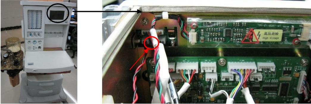
4. Disconnect the power board cable from the power signal conversion board.
