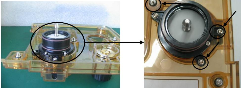
3. Unscrew the three screws of the bag/mechanical ventilation switch assembly.
