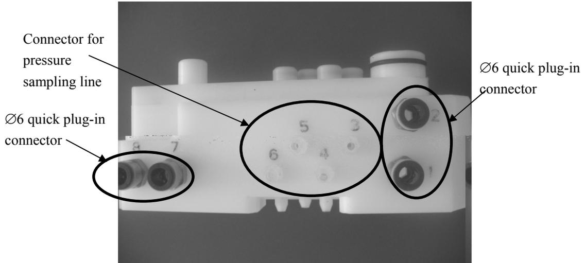
The connectors for pressure sampling lines can be connected with  $\Phi 6$  silicone tubes and the  $\varnothing 6$  quick plug-in connectors with PU tube (6X100), PU tube (6X200) and PU tube (6X300), as shown below.
