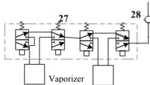
Double-vaporizer manifold 27 (or single -vaporizer manifold) is integrated with check valve 28 which prevents flushed O<sub>2</sub> and fresh gas from flowing back to the vaporizer and impairing the concentration outputted of the anesthetic agent as a result. When a double-vaporizer manifold is used, Selectatec mounting with interlocking function can prevent the user from turning on two vaporizers simultaneously.
