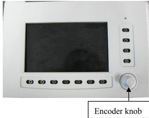
7. Loosen the nut as shown below to remove the encoder.
