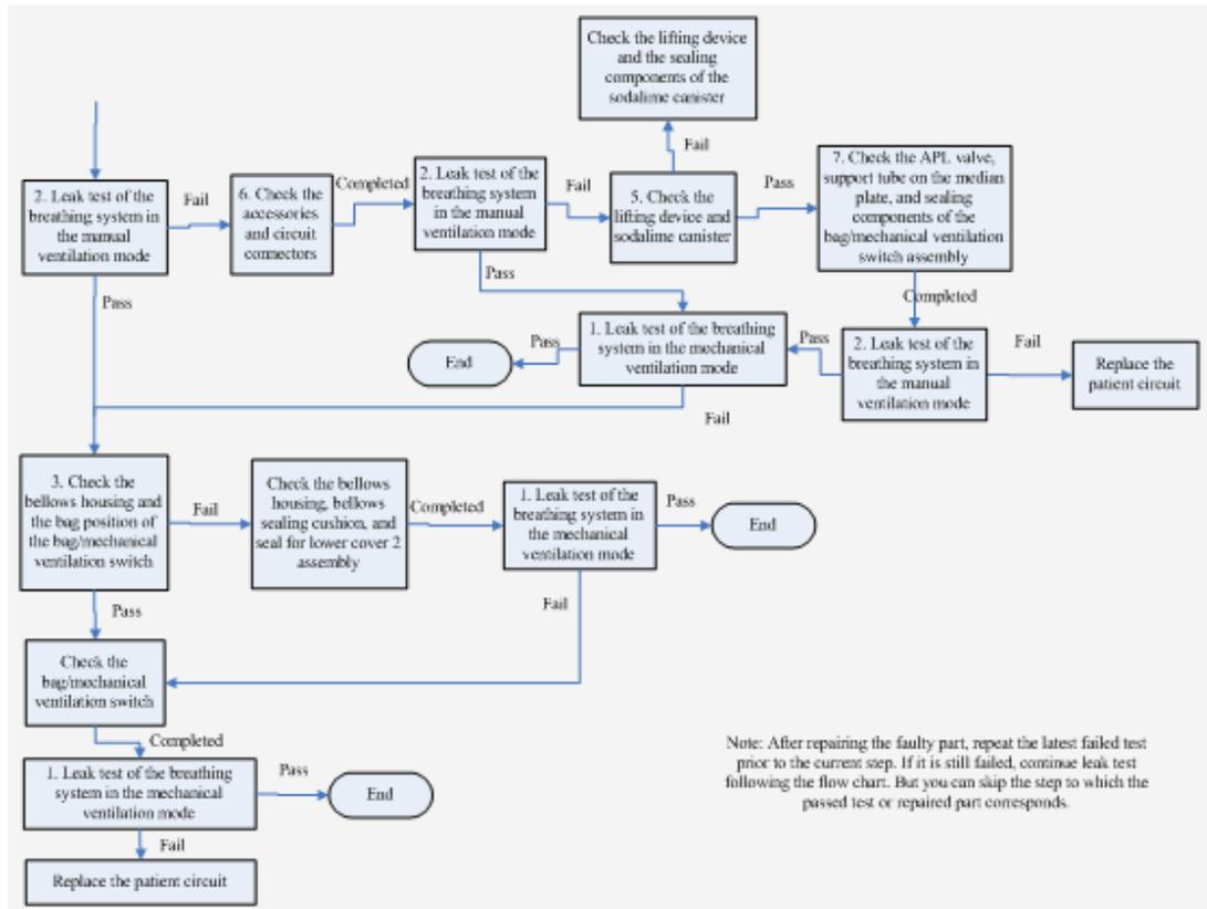
Figure d Leak test of the patient circuit
