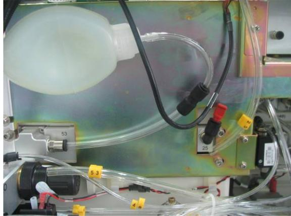
6. Release the negative pressure ball. If the negative pressure ball is fully expanded within 30s, it indicates that the rubber plain washers and seal of the tested pipeline or its contacted mechanical surface are damaged. Handle this problem as described in the troubleshooting table.
