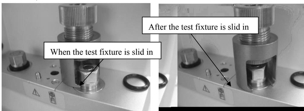
Turn the pressure head of vaporizer manifold test fixture clockwise until the bottom surface of the pressure head is in contact with the top surface of the connector of the vaporizer manifold assembly, as shown below.
