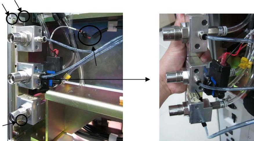
4. Unscrew the two screws on the gas supply inlet assembly to remove the O<sub>2</sub>/N<sub>2</sub>O/Air supply inlet assembly from the gas supply mounting panel (take N<sub>2</sub>O supply inlet assembly for an example).
