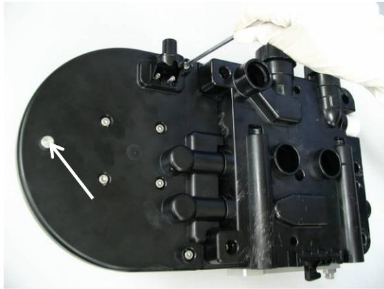
6. Turn over the circuit. Pull up to take out the upper cover 2 assembly.
