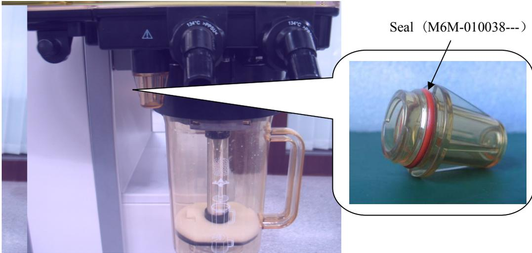
5. For WATO EX-25/30/35 anesthesia machine, as required, replace the sealing component for CO2 absorbent canister outlet (049-000154-00) and sealing component for CO2 absorbent canister (0601-20-78842) every 12 months.
