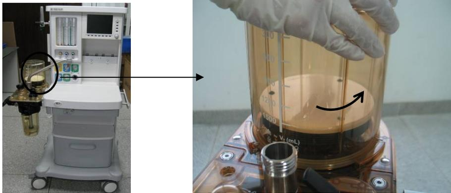
2. Lift off and remove the housing.
