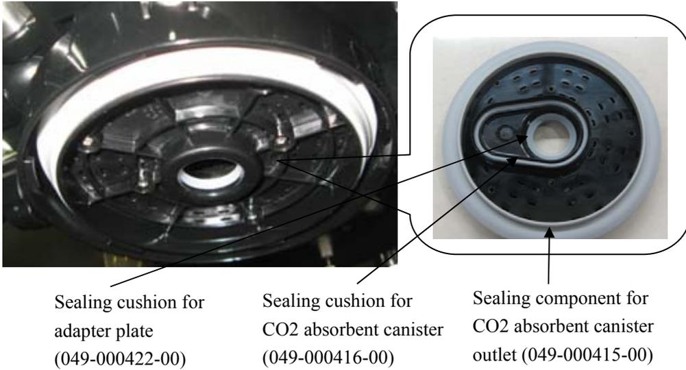
6. For WATO EX-25/30/35 anesthesia machine, as required, replace the seal for CO2 absorbent canister support (M6M-010051--) every 12 months.
