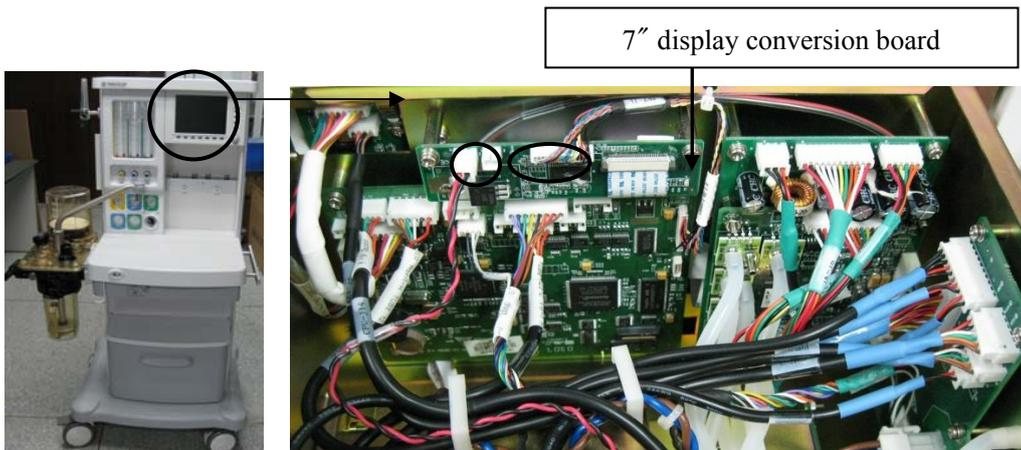
3. Disconnect the data line from the conversion board. Note: when disconnecting the data line, you must push out the black holder parallel to the conversion board.
