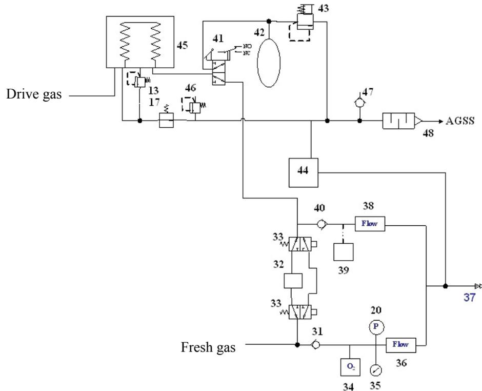
Manual and mechanical ventilation modes are selected through the Bag/vent switch. When manual ventilation is selected, the doctor presses manual bag 42 to supply gas for the breathing system. APL valve 43 adjusts the pressure inside the pneumatic circuit in case of manual ventilation. When mechanical ventilation is selected, the ventilator starts to work. It controls the drive gas to depress the bellows 45 and supply gas for the breathing system as per the selected ventilation mode.
