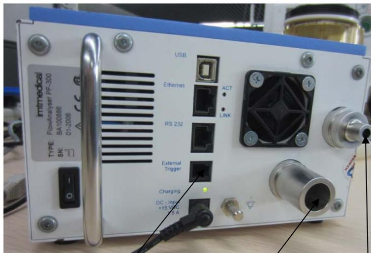
Connect calibration communication line RS232
