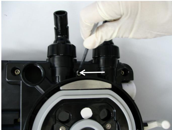
5. Remove the lifting device from the circuit.
