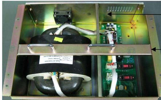
Isolation plate for the isolation transformer
