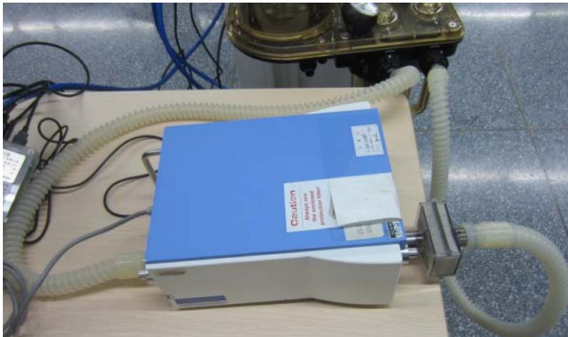
7. After flow calibration success is prompted, refer to **1.2.5 Check the Flow Sensor Accuracy** to test the effectiveness of flow calibration. In case of calibration failure, first fix the problem and then perform flow calibration again.
