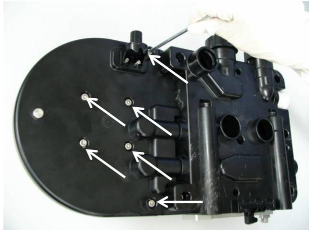
5. Loosen the nut counterclockwise as shown below.
