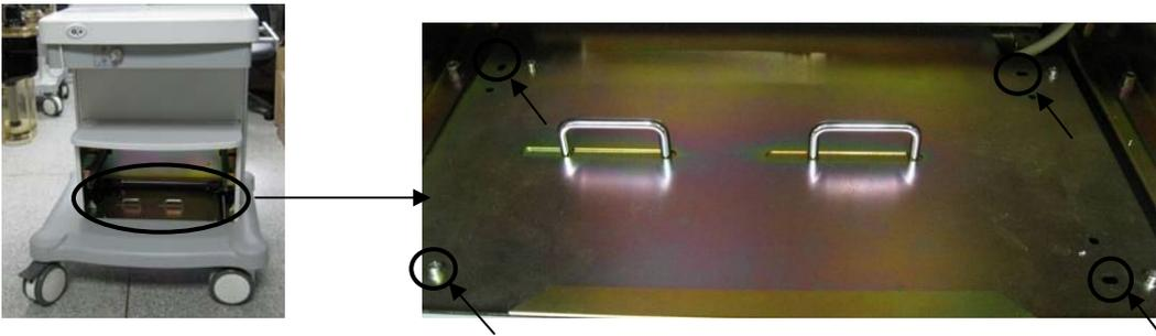
3. Disconnect the cables between the auxiliary output assembly and the isolation transformer assembly to take out the isolation transformer assembly.
