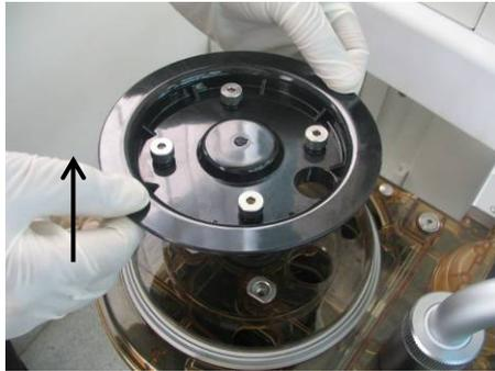
4. Take out the Pop-off valve rubber gasket and metal component.
