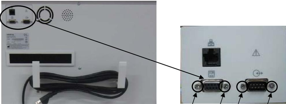
3. Disconnect the cables from the calibration power interface board and unscrew the three screws as shown below to remove the interface board.
