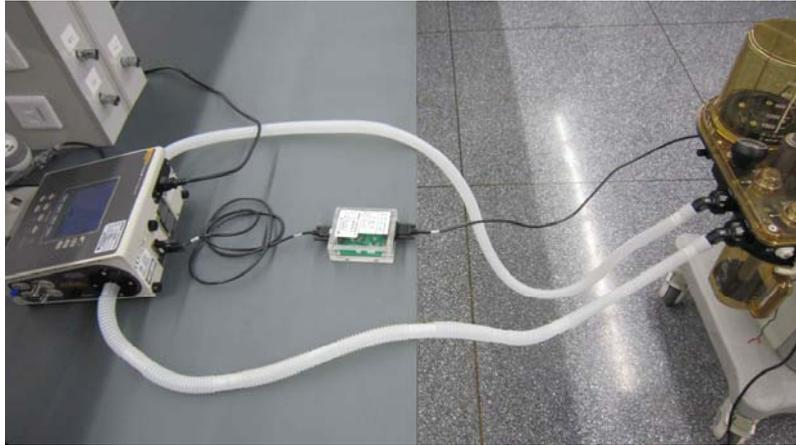
If PF300 is selected as the calibration device, connect the tube to the high flow channel of PF300 and push the button for high flow channel. The red indicator light for high flow is lit and “Flow High” is displayed in the upper left corner of the screen. Connect the protection filter at the gas inlet, as shown below. Then select [Continue].
