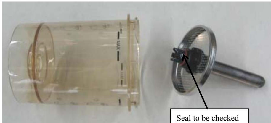
7. Check the APL valve, support tube on the median plate, and sealing components of the Bag/vent switch assembly
