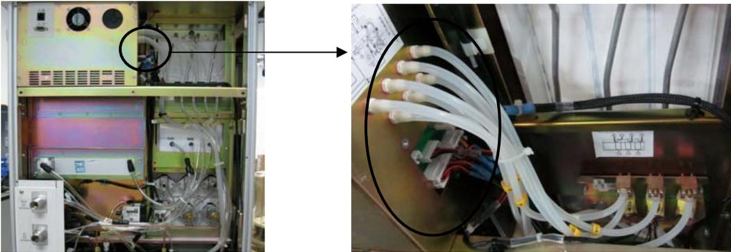
4. Unscrew the four screws fastening the ventilator assembly.
