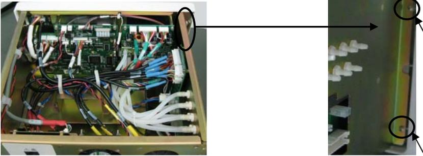
3. Disconnect the cables on the right side of the inverter and those from the keypad scanning board. Unscrew the five screws fastening the metal sheet to remove the panel assembly.
