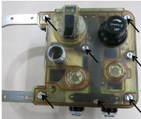
3. Hold the upper cover assembly firmly and pull up to take it out.
