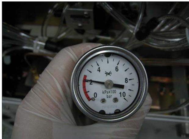
3. Turn on AIR pipeline supply. If the reading on the test pressure gauge is not within the range of  $0.2 \pm 0.05$  MPa (namely  $2 \pm 0.5$  bar), adjust the regulator to cause the reading on the test pressure gauge to reach 0.2 MPa (namely, 2 bar). For operations of the regulator, refer to section **5.3.2.4 Adjust the Regulator of the Pipeline Gas Supply Inlet Assembly**. Record the reading on the AIR pipeline pressure gauge.
