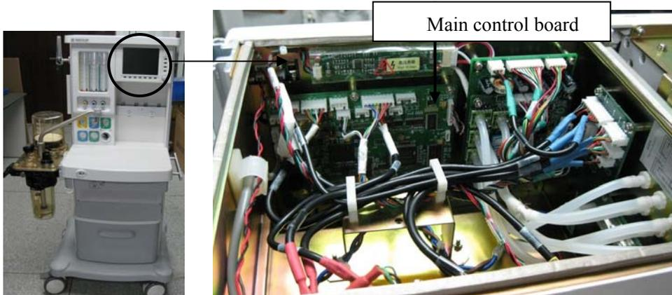
3. Unscrew the three screws as shown below to remove the main control board.
