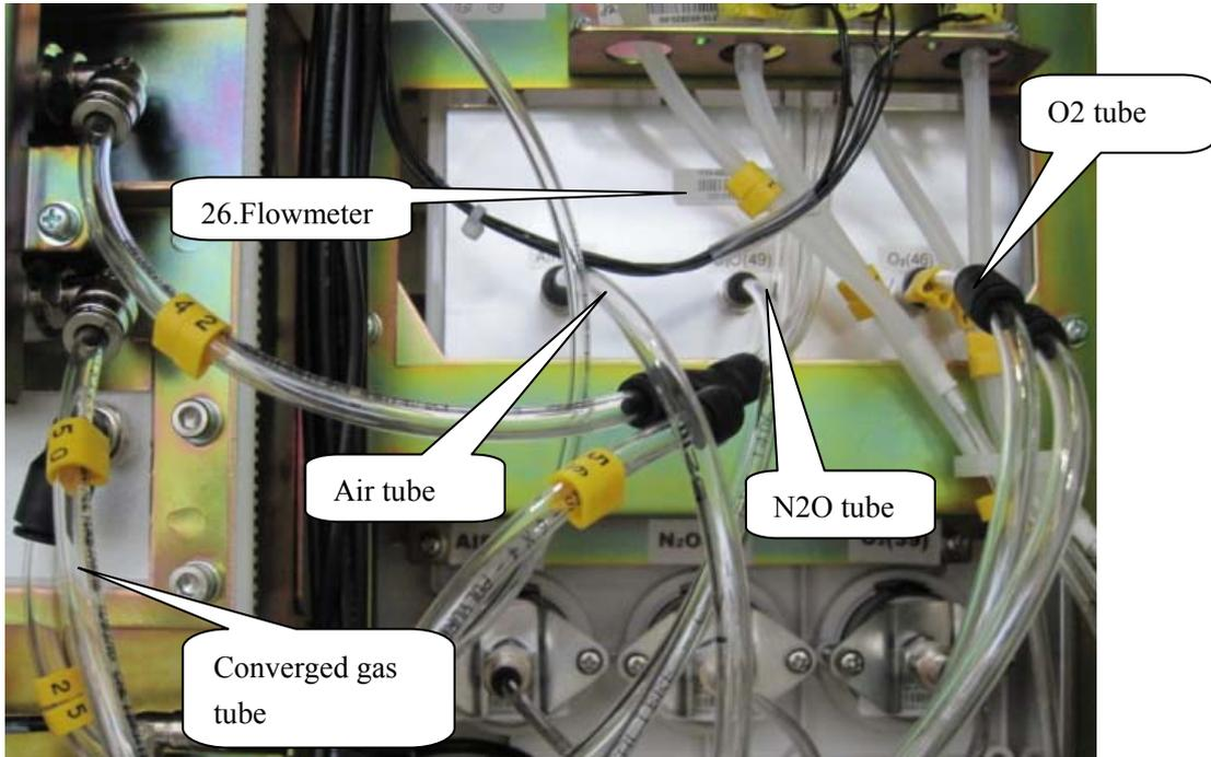
Flowmeter 26 controls gas flows. The gases passing through flowmeter 26 enter the anesthetic gas delivery system (vaporizer) as shown above.
