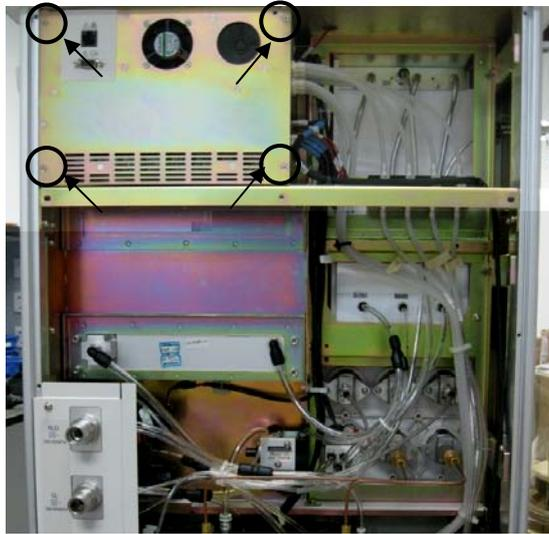
7. Unscrew the screws as shown below to remove the fan and power board respectively.
