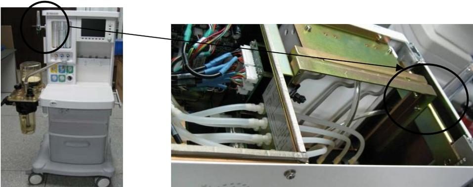
3. Pull out the upper cover plate on the left side of the machine. Unscrew the three screws to remove the auxiliary O2 supply assembly.
