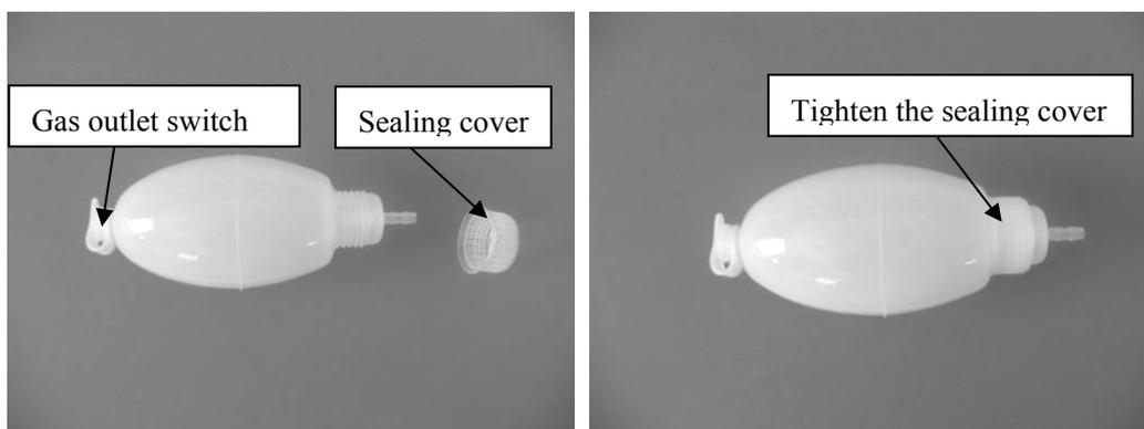
Remove the gas outlet switch to flatten the negative pressure ball. Re-install the gas outlet switch properly when performing the test, as shown below.
