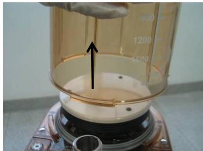
3. Remove the bellows from the bellows base.
