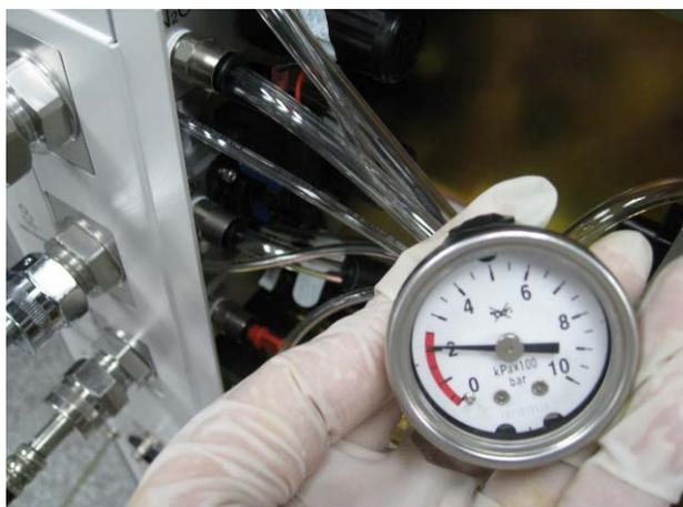
3. Turn on N<sub>2</sub>O and O<sub>2</sub> pipeline supplies. Adjust the regulator of the N<sub>2</sub>O supply inlet
