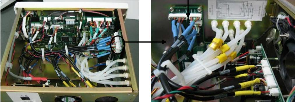
5. Unscrew the six screws as shown below to remove the power signal conversion board.
