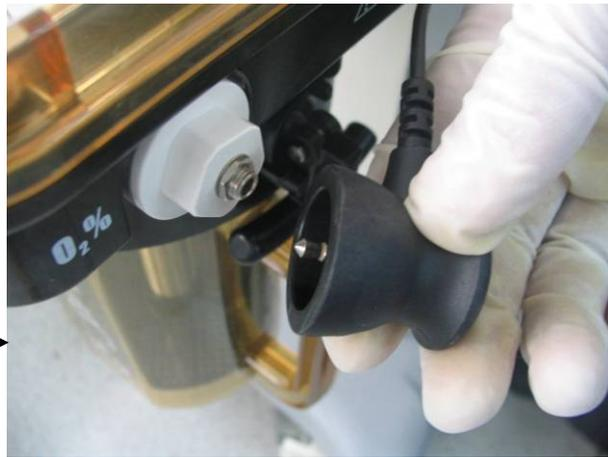
2. Turn the O<sub>2</sub> sensor counterclockwise to take it out.
