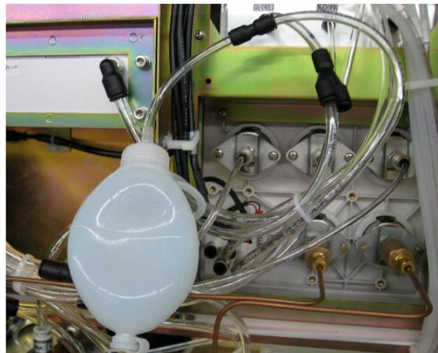
6. Release the negative pressure ball. If the negative pressure ball is fully expanded within 30s during one of the two tests, it indicates that the system switch assembly is damaged. Handle this problem as described in the troubleshooting table.
