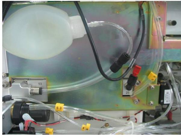
7. Release the negative pressure ball. If the negative pressure ball is not fully expanded within 30s, it indicates that the vaporizer manifold assembly is not leaky. Otherwise, check the seal between the vaporizer manifold assembly and the vaporizer (replace the seal if it is damaged), or re-install the vaporizer. Do the test again until it is passed.
