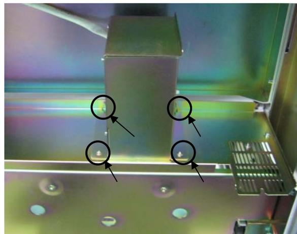
2. Unscrew the four M3x8 pan head screws to open the heating control box assembly.
