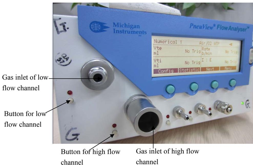
Gas inlet of low flow channel
