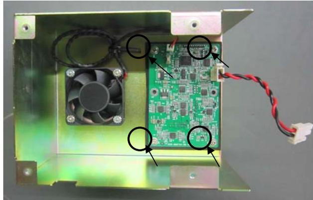
4. Unscrew the four M3x8 pan head screws to remove the power board.
