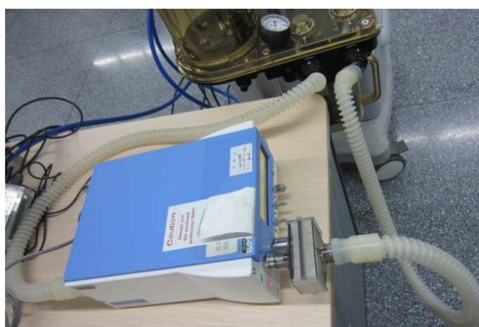
Figure b: low flow connection, with protection filter
