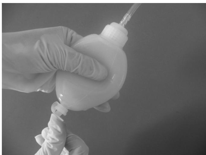
Before using the negative pressure ball, make sure that it is not leaky. Check if the front sealing cover is tightened. Then flatten the negative pressure ball to remove the gas inside. Install the gas outlet switch properly. Block the front gas inlet with your hand to release the negative pressure ball main unit. Visible expansion of the ball cannot be seen within 30 seconds. Otherwise, replace the ball.
