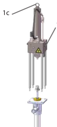
Remove oscillating cylinder Fig. 28
