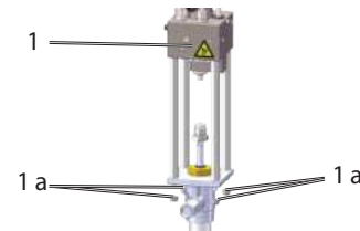
Loosen the nuts of the distance rods Fig. 37
