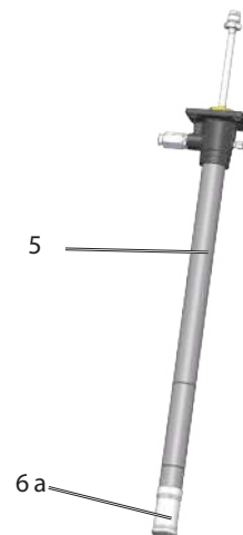
Remove oscillating cylinder Fig. 28
