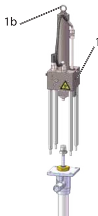
Remove oscillating cylinder Fig. 10
