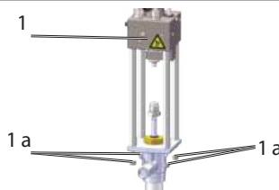
Mount oscillating cylinder Fig. 40
