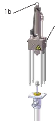
Remove oscillating cylinder Fig. 38
