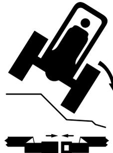
THIS TRACTOR MAY TIP OVER UNEXPECTEDLY AND QUICKER THAN AN OPERATOR IS ABLE TO JUMP FREE.
