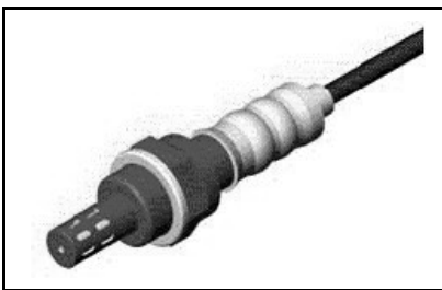
Figure 3-82. Heated Exhaust Gas Oxygen Sensor (HEGO)
