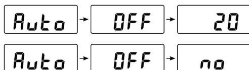
The user can toggle the selection by pressing CAL/SELECT or move to the next step with CFM/SETUP.
