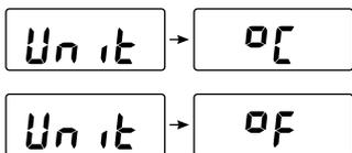
Press CAL/SELECT to toggle the selection and CFM/SETUP to exit the menu selection mode and return to normal measurement mode.
