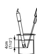
**Note:** The electrode should be submerged approximately 4 cm (1 1/2") into the solution. The temperature probe should be located close to the pH electrode.
