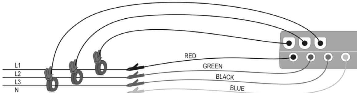
Instrument connection in a three-phase 4 wire system
