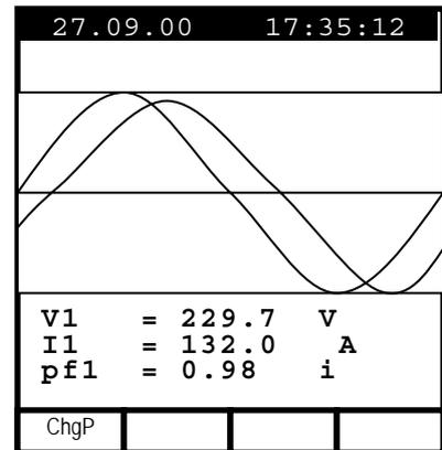
Example of screen in "4 wires" three-phase mode
