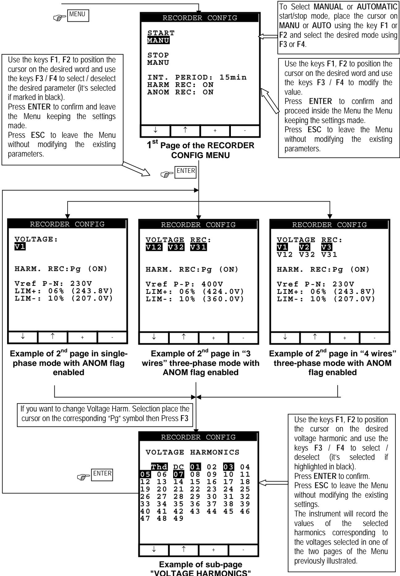
Use the keys F1, F2 to position the cursor on the desired word and use the keys F3 / F4 to modify the value or select / deselect the desired parameter (it's selected if marked in black). Press ENTER to confirm. Press ESC to leave the Menu without modifying the existing settings.
