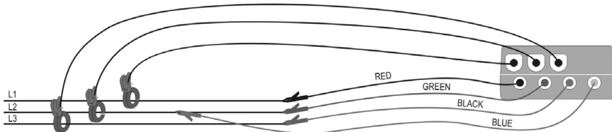
Instrument connection in a 3 wires three-phase system
