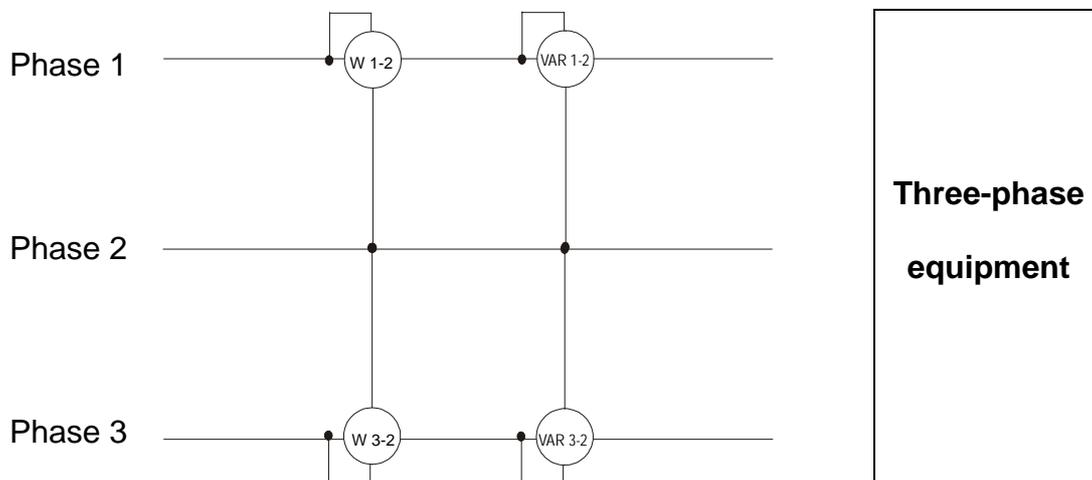
In this case the potential of one of the three phases (for example, phase 2) is taken on as reference potential. The total values of the active, reactive and apparent power are expressed as sum of the indications of the couples of Wattmeters, VARmeters and VAmeters.
