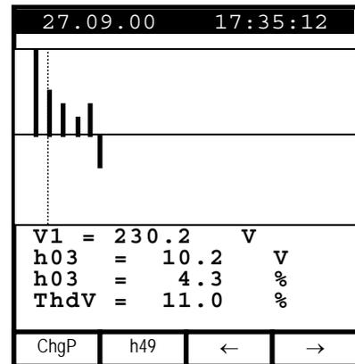
Example of screen in "4 wires" three-phase system
