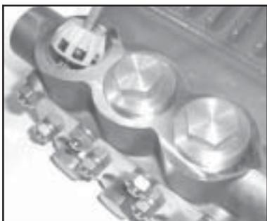
14. Next, place valve assemblies (46A) into manifold after first lubricating the o-ring (44A). Seat firmly into manifold.
