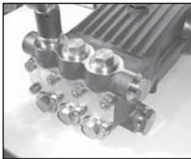
15. Replace plug with o-ring (48, & 48A) and tighten to 160 ft.-lbs.
