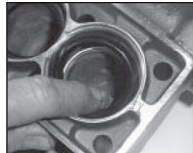
9. Lubricate weep seal (36). Place, weep seal (36), and pressure ring (36A) into the seal sleeve (35). Assemble the o-ring (35A) onto seal sleeve and lubricate.
