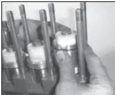
11. Press seal sleeve assembly into the manifold and seat firmly. Put the support ring (41) on plunger with v-side facing the manifold.
