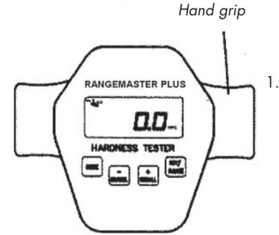
1. Stand comfortably with your arms directly over the tester. Take a firm hold of the hand grip and push down slowly until you feel the diamond touch the test block.
