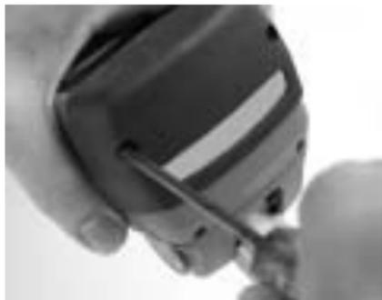
**B.** Open the battery pack by removing the cover.
