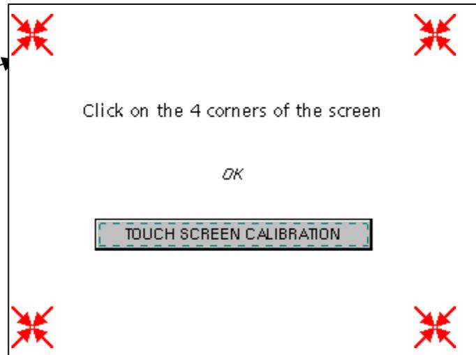
Use the stylus to point at the centre of the 4 patterns displayed on the screen. Validation of the input is indicated by modification of the pattern.
