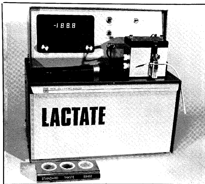
Figure 1. The YSI 23L Lactate Analyzer
