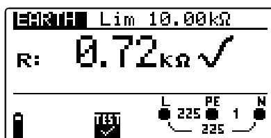
Figure 5.10: Example of earth resistance measurement result
