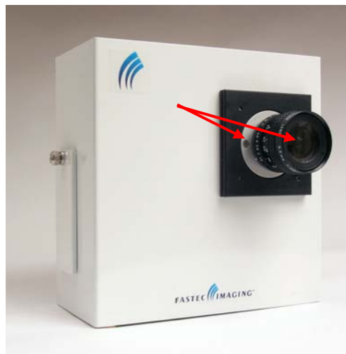
Figure 2-3: Back-Focus Ring Retaining Screws
